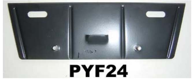
PYF24 ..... 1965 FRONT LICENSE BRACKET Includes 2 bumpers and mounting hardware to bumper.
