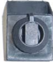
RPT35G.....1964-72 REAR QUARTER PANEL RUBBER VENT This is a rather large square hooded rubber grommet plug found under the rear quarter panel of most GTO's.
