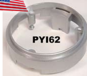
PYI62 ..... 1968 SPORT WHEEL COLLAR Originally die cast, these repro's are molded plastic. PAINTED SILVER. PYI64 ..... 1969-70 SPORT WHEEL COLLAR Nice true satin chrome plated plastic.
