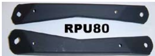
RPU80.....1964-67 REAR BRACES These braces were originally installed on just manual trans cars. They prevented wheel hop. They bolt from the frame mount of the lower control arm to the frame mount of the upper control arm.
