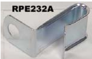
RPE232A ..... 1964-67 STARTER WIRE RETAINER Mounts on the valve cover bolt. All exc. 67 HO/RA. Keeps wire away from head bolt. Painted engine color 1964-65 models.
